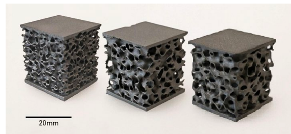
Fig. 2: Support-free 3D-printed titanium samples with different generation parameters.
