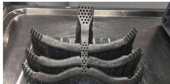
Fig. 1: ALM Hemi-Thoracic cage in Ti6Al4V.
